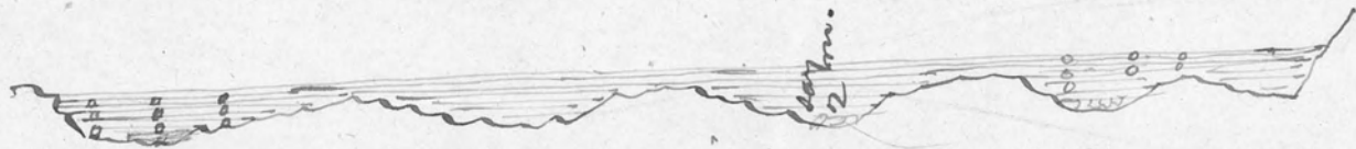
Sketch of Orb-dam - across an outl. of irregular bottom - Or. of a rough-stone embankment - as the case may be.
